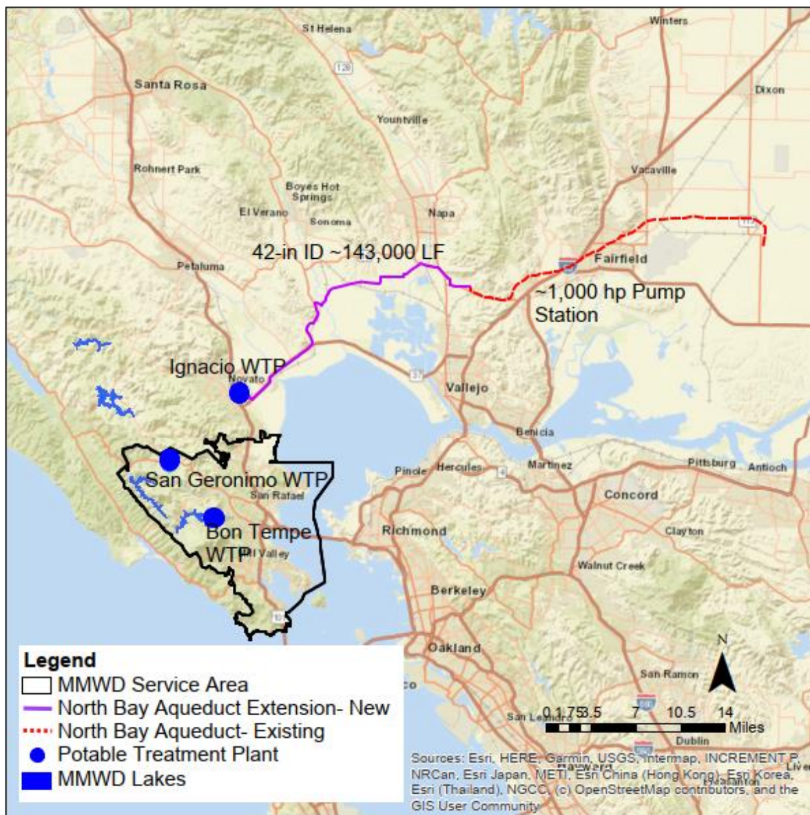
Figure C-16. North Bay Aqueduct Intertie Concept
