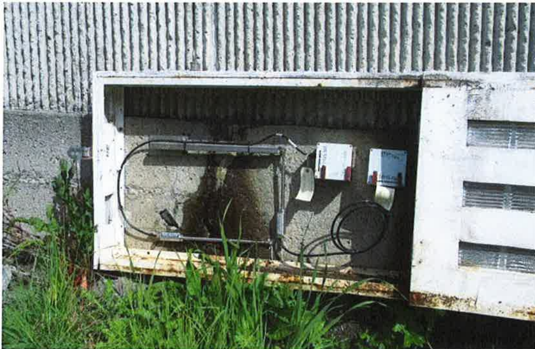
The raised portion of the spillway, above, and the extensometers monitoring movement along a crack through the spillway foundation, below. The location of the instrumentation is circled in the top photograph.
