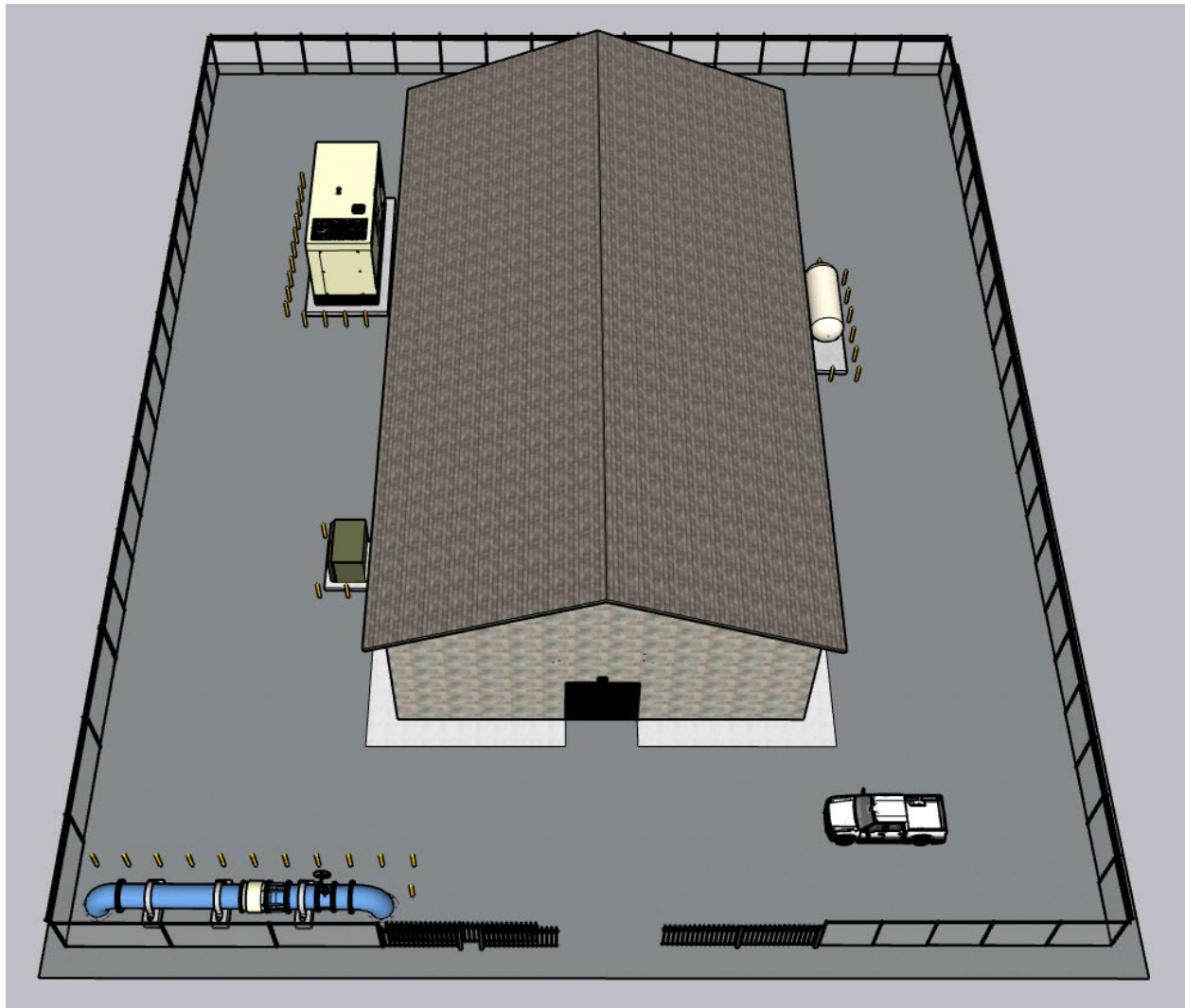
Figure 3.15 PETA-3 Pump Station B Site Layout
