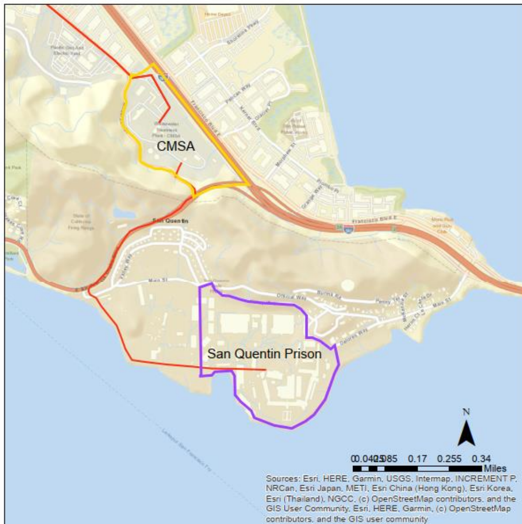
Figure C-21. Non-potable recycled water system conceptual map: CSMA to San Quentin prison (from Water Resources Plan 2040, 2017).
