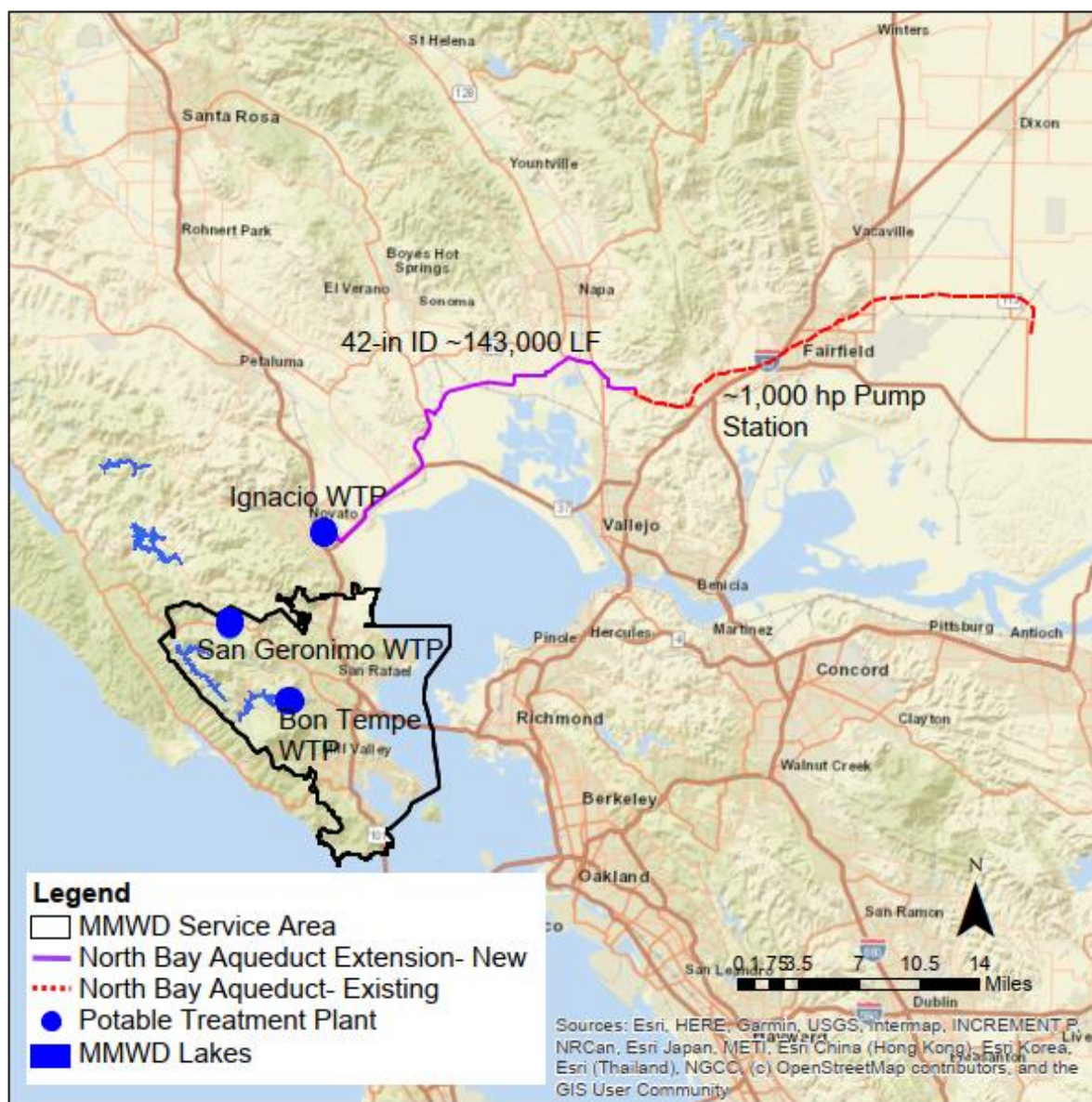
Figure C-16. North Bay Aqueduct Intertie Concept
